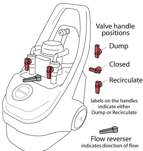
1. Leave the pump tank cap loose, or on by no more than one turn if water splashes whilst flushing / descaling (to allow gas to escape).
