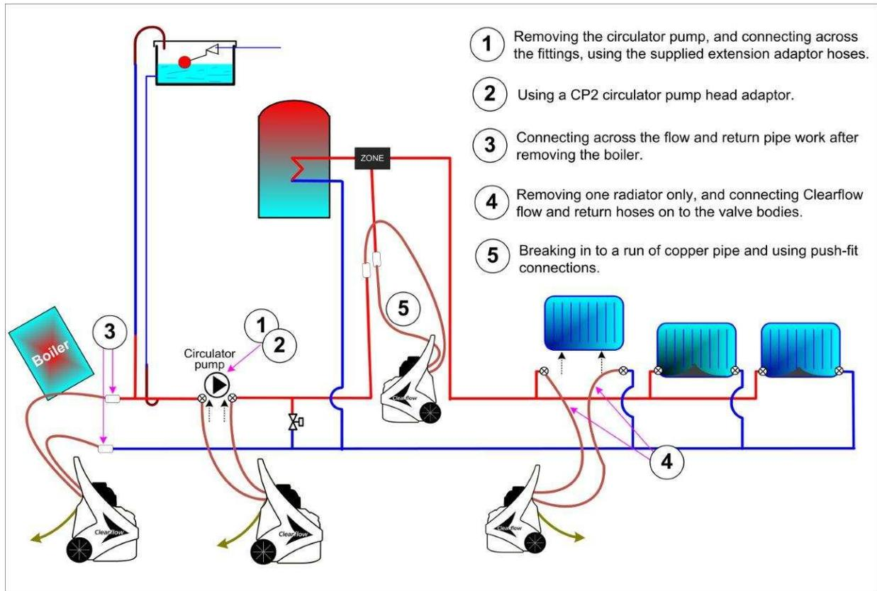
The connection point for the flushing pump may vary depending on the system to be cleaned, and the availability of suitable connection points.
