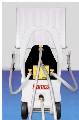
2c. Across the "tails" of a radiator (having drained and disconnected the radiator) using appropriate 1/2" or 3/4" BSP adaptors to connect to the valves. The radiator valves should be closed to isolate the flushing pump from the system until power flushing is commenced.
