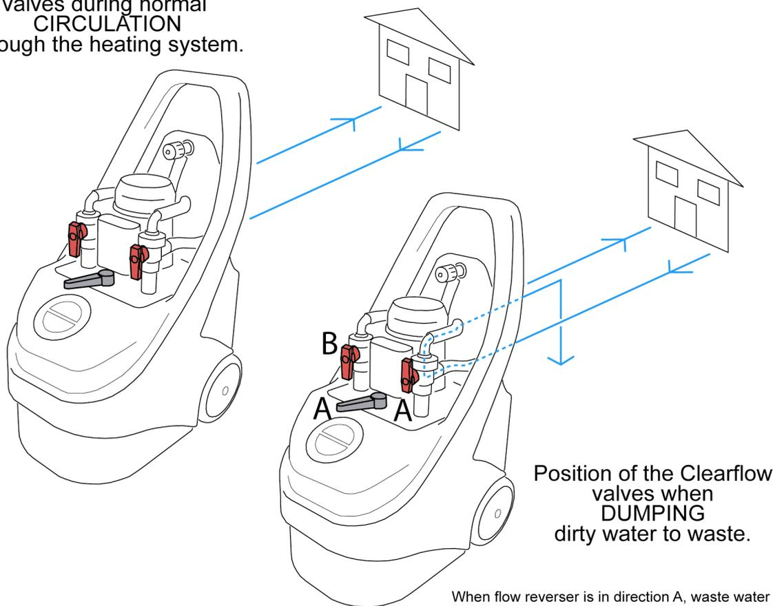
Position of the Clearflow valves when DUMPING dirty water to waste.
