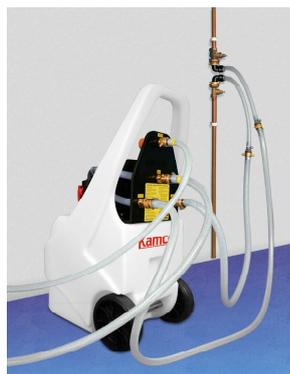
A pair of 0.5 metre long adapter hoses, enabling the pump to be connected across the 1 1/2" unions, are supplied as standard. When used, these are screwed directly onto the 3/4" female brass hose adaptors of the flow and return hoses, giving a total hose length of 5.5 metres.
