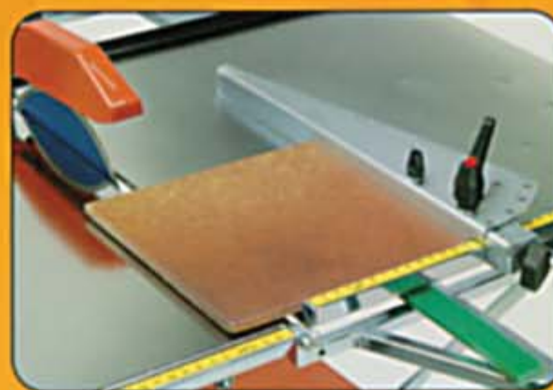
Direct reading of the cutting measure.
