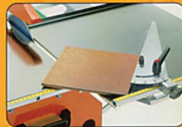
Direct reading of the cutting measure on diagonal.
