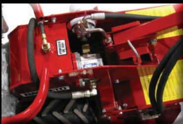
All hydraulics are easily accessed for maintenance and repair
