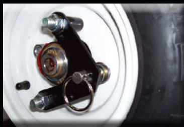
Hubs unlock to free-wheel the tiller when the engine isn't running
